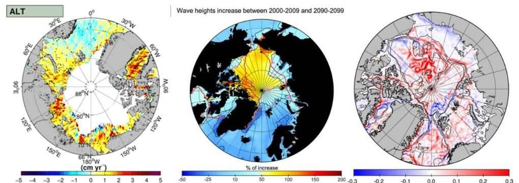
Figure 7: Observed trends in significant wave heights 1992–2014 from Stopa *et al.* (2016) (a) along with the projected significant wave heights increase (b) and increase in the speed of the ocean surface currents (c) from the 2000s to the 2090s. (From Aksenov *et al.*, 2017.)
