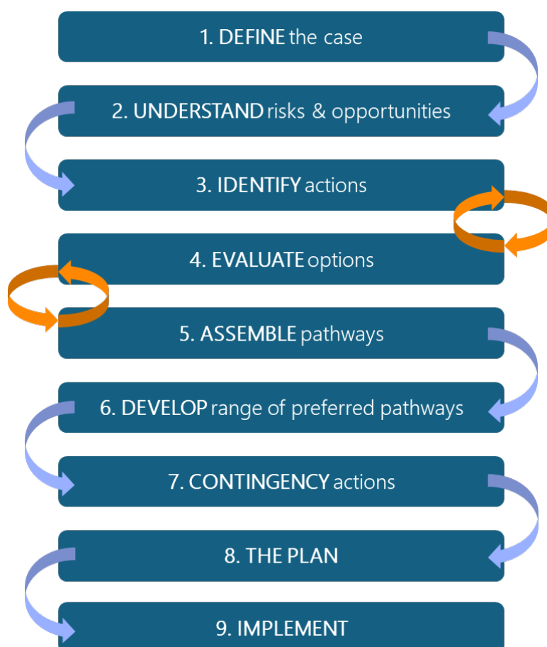
Figure 9. Steps to develop climate change adaptation pathways. The orange circular arrows indicate points for reassessment and where to integrate quick low-regret, short-term actions that have well-evidenced benefits, with long-term options to adapt, if necessary (BSI, 2021).
